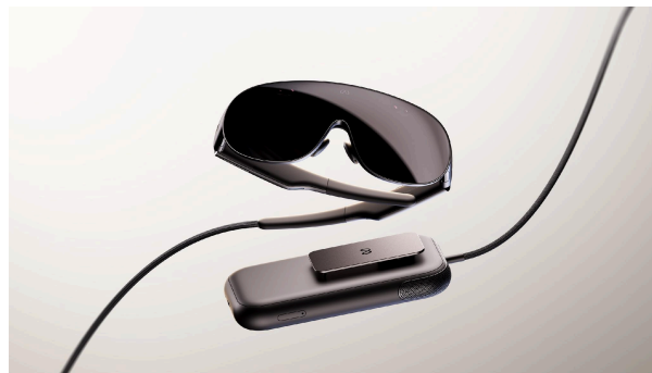
Meta VR Glasses with the compute puck and its cable. Image courtesy of Meta.
