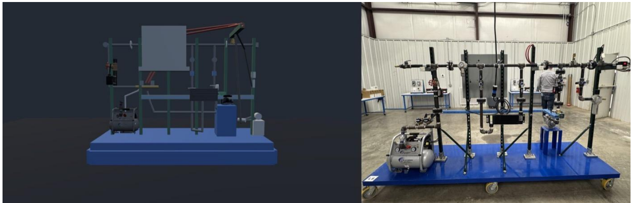
Figure 2 — the demonstration twin (left) against the machine (right), same viewpoint. Real components where evidence supports them; badged primitives where it does not.
