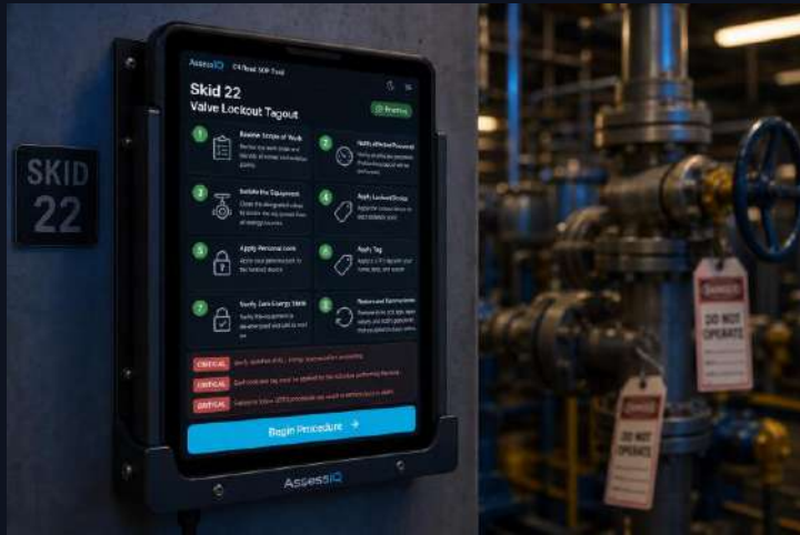
Skid tablet showing SOP card · 8 steps with criticality ruggedized tablet on stand, current step highlighted
